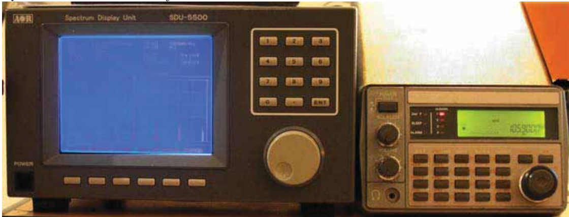
The finished mod showing the broadcast band 9Mhz span
