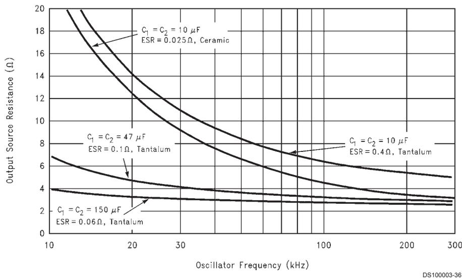
FIGURE 3. Output Source Resistance vs Oscillator Frequency
