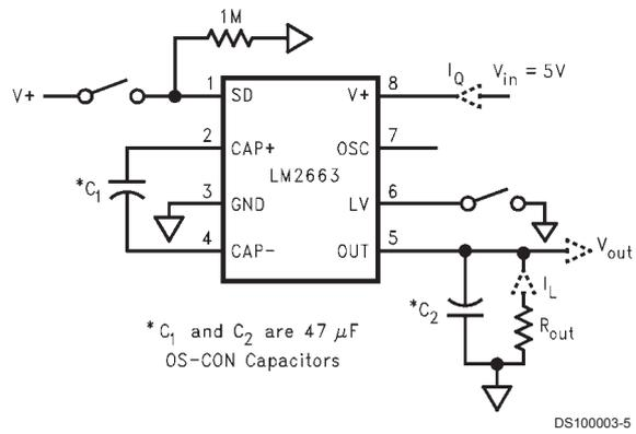
FIGURE 1. LM2662 and LM2663 Test Circuits
