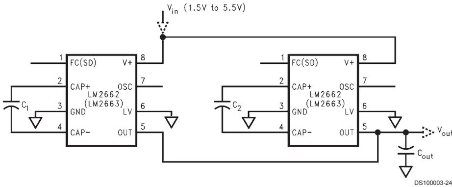
FIGURE 4. Lowering Output Resistance by Paralleling Devices
