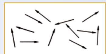
Figure 2 Ferrite in Unmagnetized state
